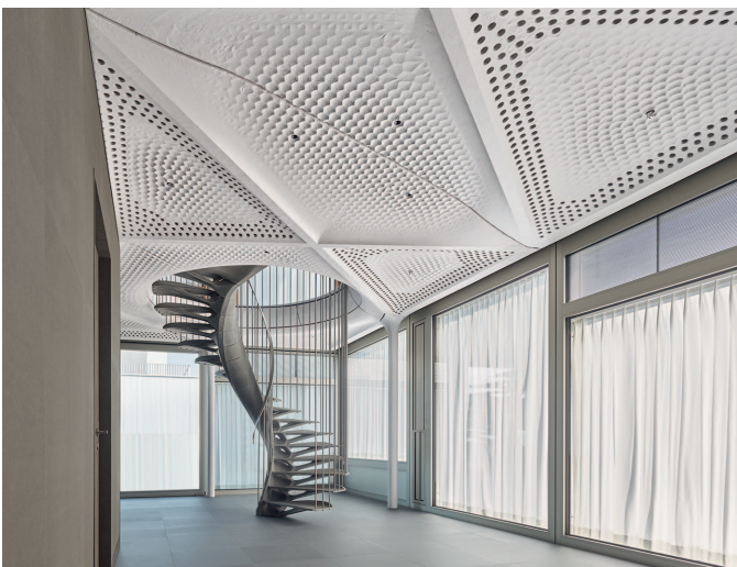
Fig. 2 Innenraum STEP2 mit IPF-Decke, Cadenza-Treppe und «Closed Cavity»-Fassade. Inside of STEP2 with IP Floor, Cadenza stairs and closed cavity façade. (© Zooney Braun)
